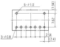
UM1L-D type (Double winding latching type)
